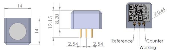
All dimensions are in mm with a tolerance of  $\pm$  0.15 mm unless stated otherwise
